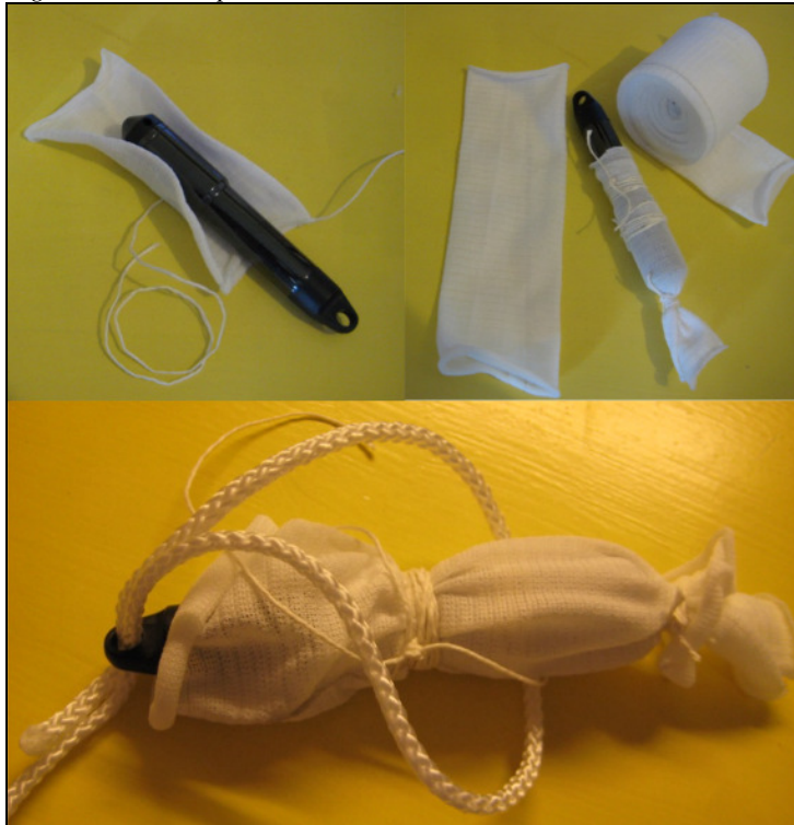
Figure D3: Protection of a Diver against sand particles
