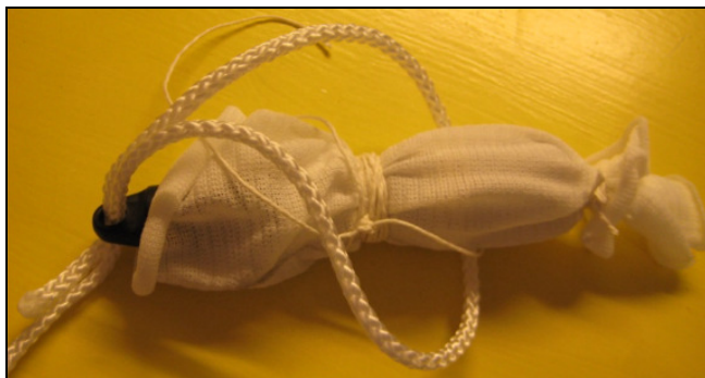
Figure 24: Protection of a CTD-Diver against sand particles
