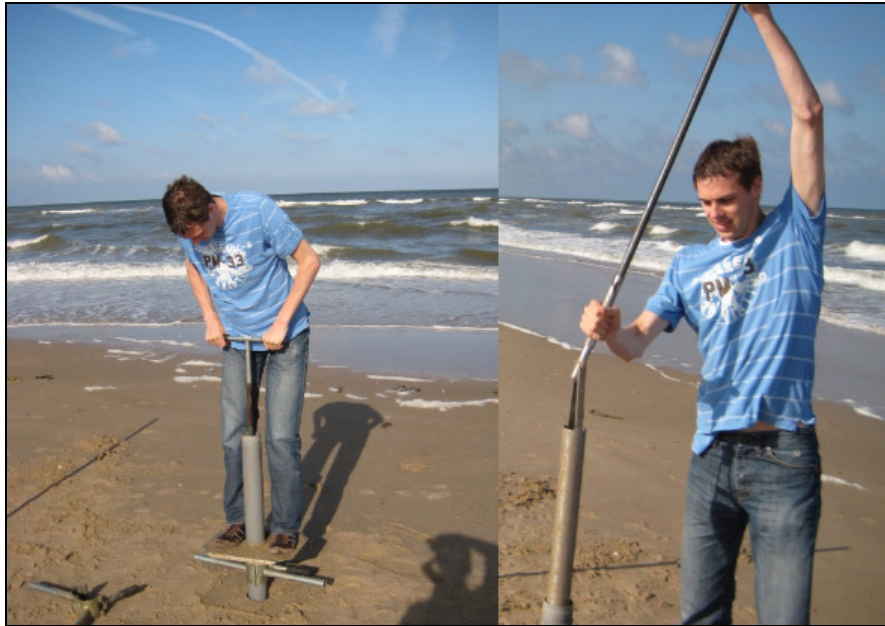
Figure D4: Operation of a pulse drill
