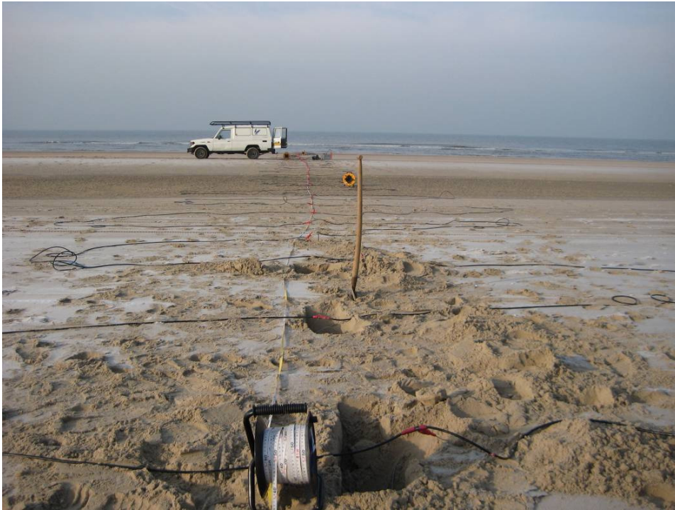
Figure 3.4 Set up of a CVES perpendicular to the shore with a profile length of 80m. On the relatively dry part of the beach, the electrodes were placed deeper (0.5m) in the sand to cope with possible electrode contact problems.
