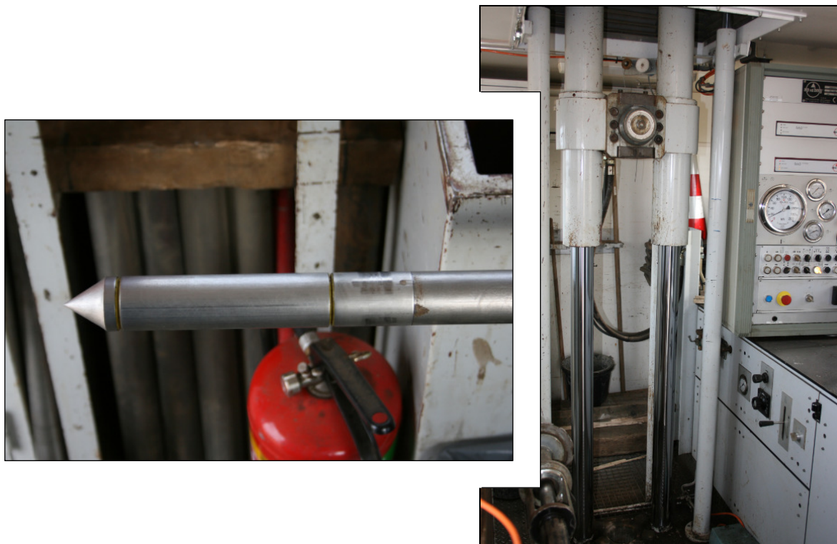
Figure 3-11 Cone penetration tests to study the conditions of the subsurface
